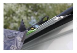
2. Attach the canopy to the vehicle using the twin piping (4mm x 6mm).
